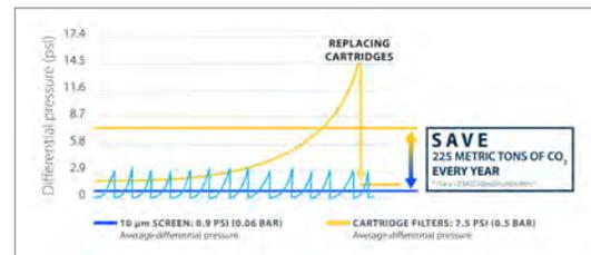
**FIGURE 3.** Head loss profiles of cartridges and automatic screen.
