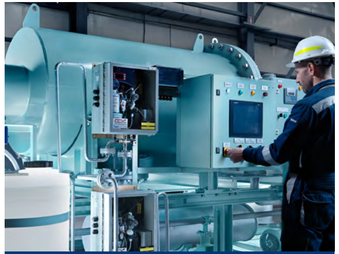
Filtersafe filter within an ERMA FIRST BWMS installation
