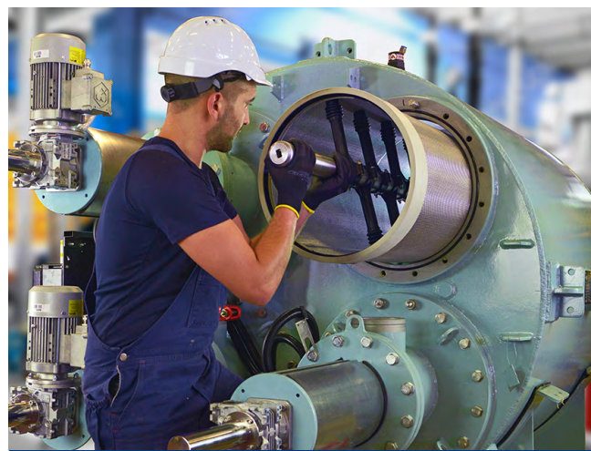
Installing our patented nozzle ® screen cleaning technology within a BSE Multi-Screen filter.
